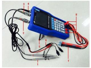
Note: picture 1-3 is for single channel oscilloscope connected input, dual-channel picture 1-3 oscilloscope connected input is from left to right CH1 and CH2 and CH3, OUT (i.e., channel 1, 2, digital channel and signal generator output)
